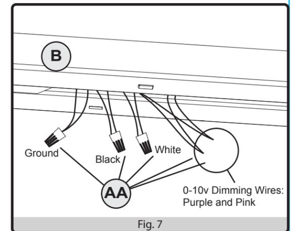
8. Re-connect the connectors between the housing base (B) and LED cover assembly (A).
