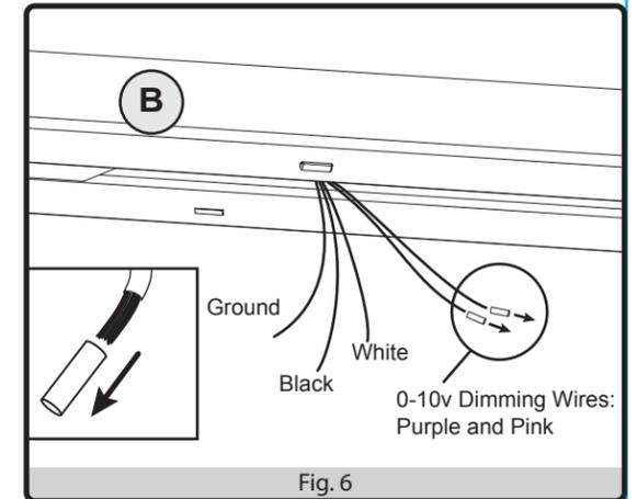
7. Reconnect ground (yellow & green) and LED wires (white & black) before reconnecting channel cover **WARNING:** If there is no ground supply wire, stop installation and consult a qualified electrician.
