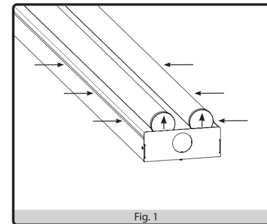
2. Disconnect ground (yellow&green) and LED wire (white) and (black) and set channel cover aside. Place channel cover in safe location.
