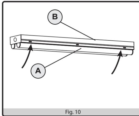
11. **Row Connector:** Insert row aligner into the slots provided at the end of the main channel housing. Ensure locking tabs are facing the locking tab hole provided in the main housing body. Slide row aligner tab into slot until an audible click is heard.
