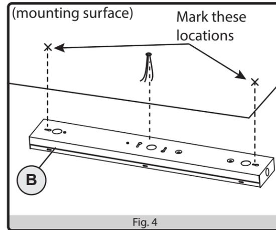
4. **DRYWALL MOUNTING:** If the mounting holes go through drywall without a stud, drill four small pilot holes using a 1/8-in. drill bit (not included), and install drywall anchors into the holes with a hammer (not included).
