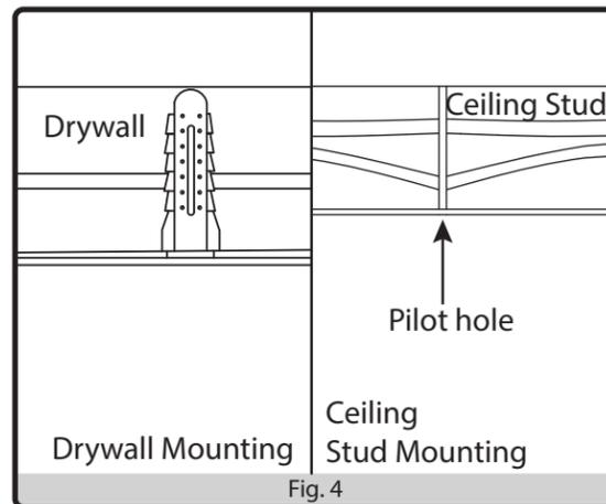
5. Feed the supply wires from the mounting surface through the knockout hole on the housing base (B). Guide the heads of the two wood screws into the keyhole slots and slide the housing base (B) in the direction such that the wood screw heads rest over the narrow part of the keyhole slot. Ensure that the fixture is supported and tighten the two wood screws (DD NOT included) until the fixture is secured to the mounting surface.
