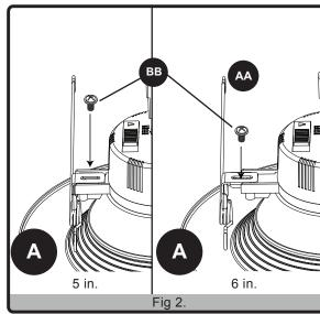
3. Squeeze the two sets of spring clip arms up towards each other and proceed to the next step to install the downlight into the can.
