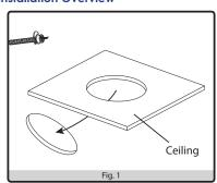
Installation can be made through cutting in a new ceiling or into an existing fixture with a through-hole (reflector needs to be removed first)
