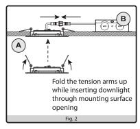
Mount the junction box (B) and make all electrical connections, pass the downlight (A) through ceiling surface and secure as shown.
