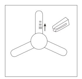
Slide the clip in small increments away from the center of that blade. Move the clip, operate the fan, then move it again until you eliminate as much wobble as possible.
